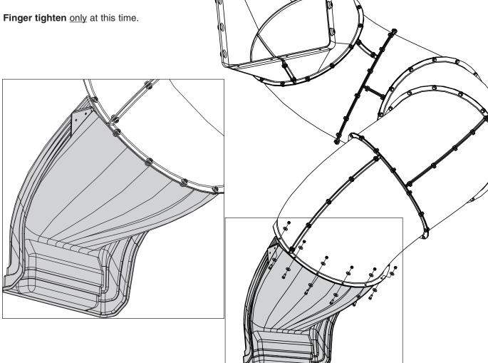
At this time use a 1/2" socket and wrench to tighten all the nuts and bolts that have been finger tightened in Steps 4 through 10 while making sure flanges are relatively flush with each other.
